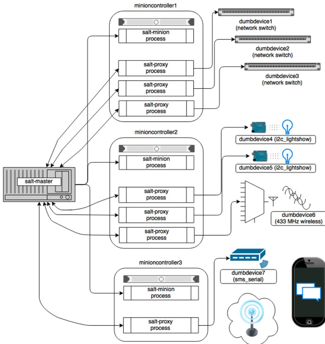
The key thing to remember is the left-most section of the diagram. Salt's nature is to have a minion connect to a master, then the master may control the minion. However, for proxy minions, the target device cannot run a minion.
